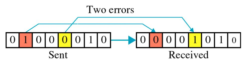
The term **burst error** means that two or more bits in the data unit have changed from 1 to 0 or from 0 to 1.
