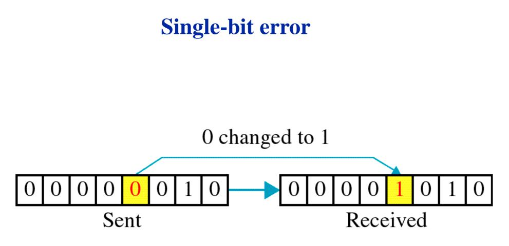
**Single bit errors** are the **least likely** type of errors in serial data transmission because the noise must have a very short duration which is very rare. However this kind of errors can happen in parallel transmission.
