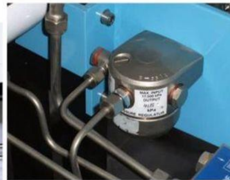
Fig 2: Pressure regulator positioned under the anaesthetic machine tray
