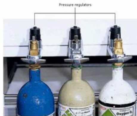
Fig 1: Gas cylinders attached to pressure regulators at the back of the
