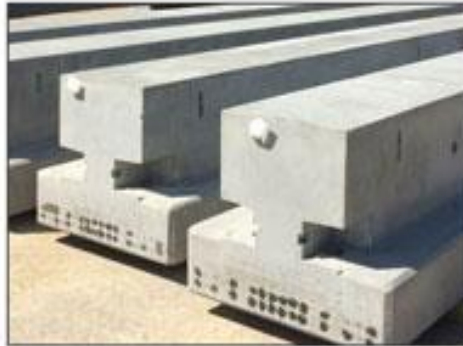
PRECAST CONCRETE BEAM
