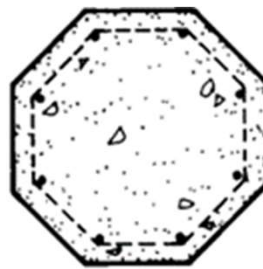
PRECAST CONCRETE PILE
