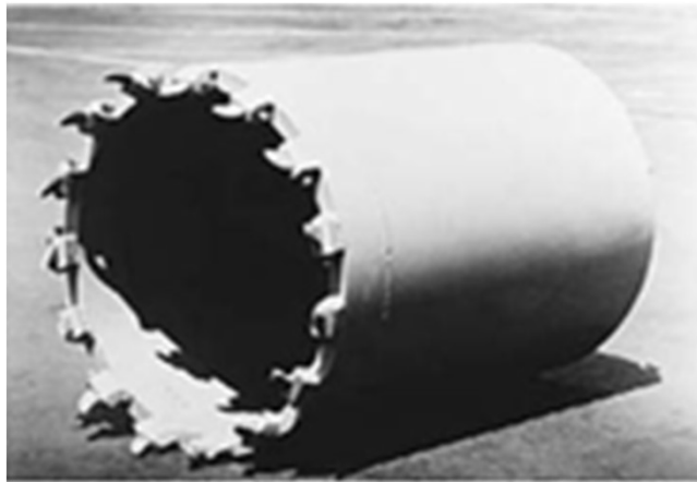
Fig.4.21: Large auger drills are used for drilling caissons
