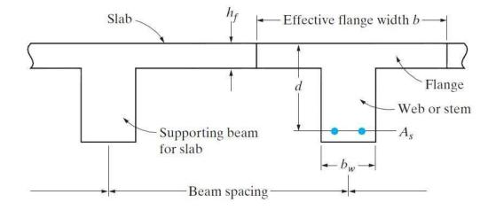
Figure 13 T-beams [4]
